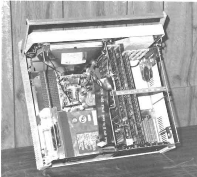
The completed unit with all supplied circuit boards in place. Note the H-8 style circuit board retaining bar. Also note the CRT contact fingers mentioned in the text.
