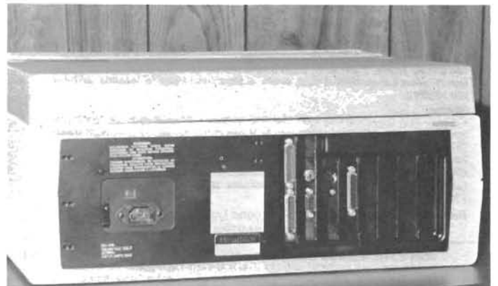
The H-161 backpanel showing the two RS-232 Ports, the Composite and RGB Video connectors, the Keyboard connector and Parallel Port connector.
