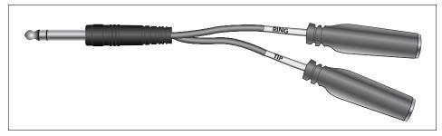
This type of adapter allows you to use the Headphone jack as another pair of line outputs. The tip and ring of the headphone plug are split off into separate outputs.
