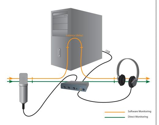
Direct Monitoring allows you to listen to the **direct** sound of your instrument during recording, without the delay incurred by going to the computer and back.
