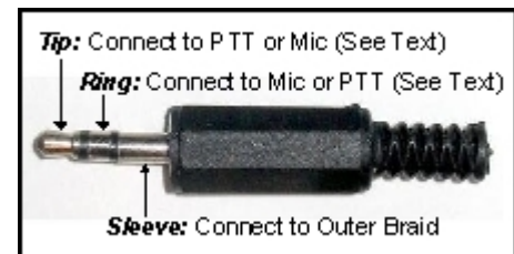
Fig 2: Microphone Plug Connections
