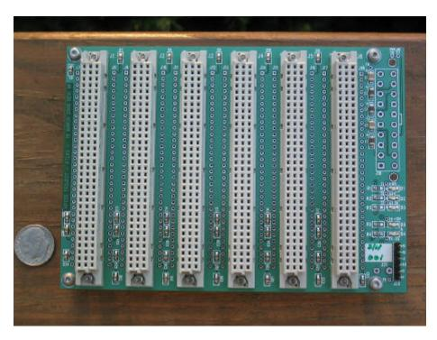
Assembled board with serial no. 001 (photo Phil Covington, N8VB) Please note that the ATX connector is not in place yet
