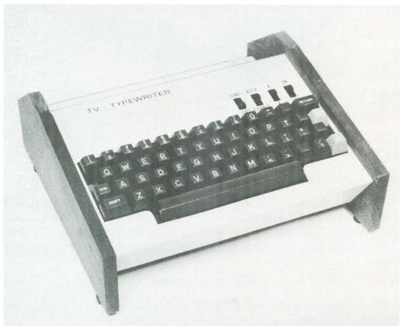
Fig. 1-3. The tvt-3 uses CMOS and RAMs; it is 8-bit microprocessor DMA compatible.
