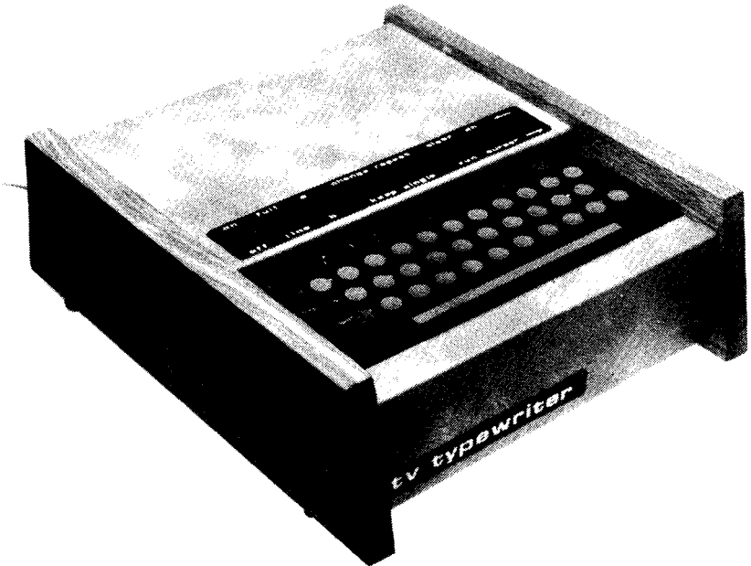
Fig. 1-1. The tvt-1 using TTL and shift-register memory.
