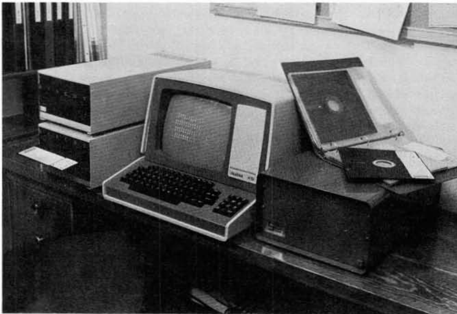
FIGURE 2-4 photo: PAWEKPIX A component system. From left to right: two 8-inch drives, terminal, and S-100 processor cabinet. This book was written on the system shown.
