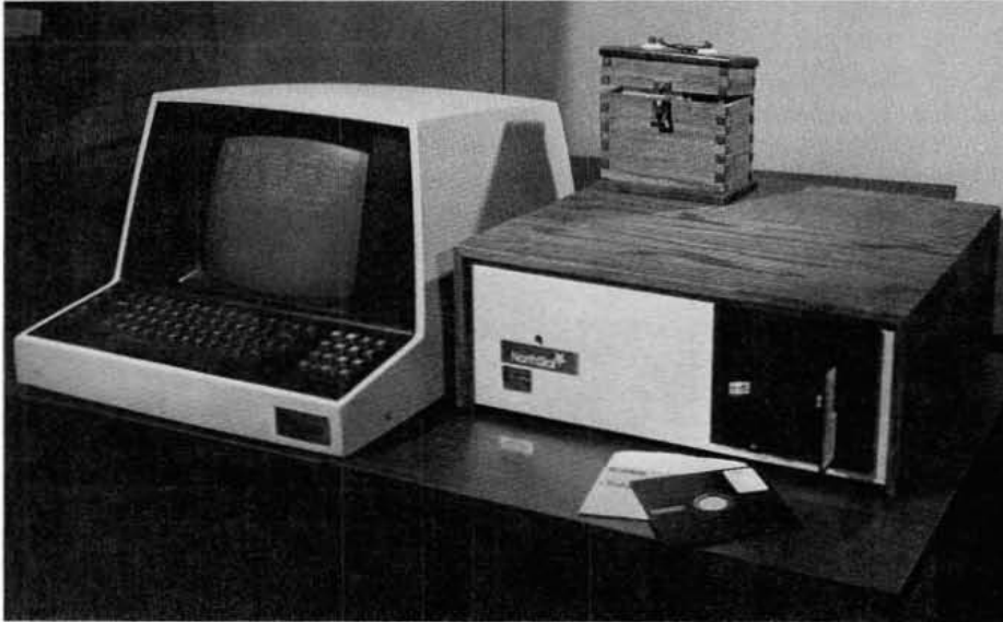
FIGURE 2-3 photo: PAWEKPIX This system, like that in Figure 2-2, puts electronics and drives in a single cabinet. In this case the drives are of 5-inch diameter, and the electronics are organized around the S-100 bus.
