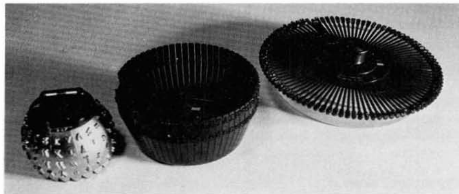
FIGURE 2-11 Three ways of doing letter-quality printing: the familiar ball, the thimble, and the daisy.
