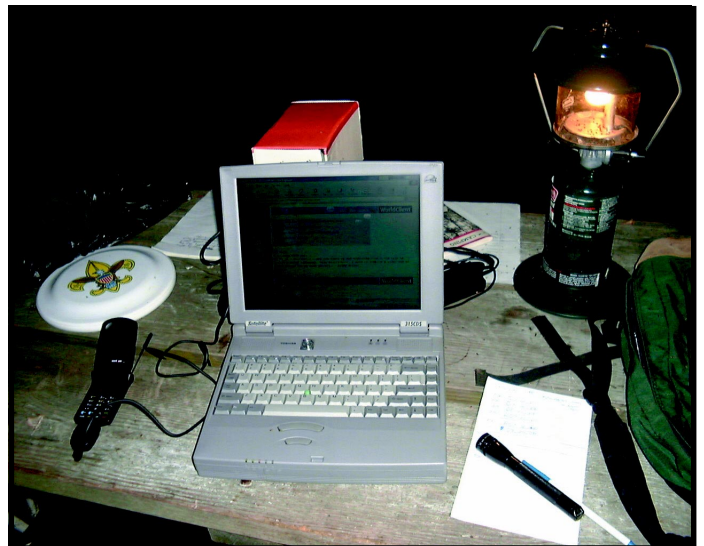
Photo 1— My StarTAC is connected to a Toshiba laptop via Motorola's connectivity kit. Internet Explorer dials out to the cell phone connected as an external modem. My ISP gets me on the Internet where I can surf or connect to get my e-mail.
