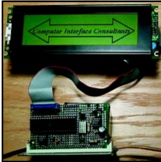
Photo 2 —My prototype was built on a DonTronics SimmStick protoboard, shown plugged into the matching DT003 motherboard.
