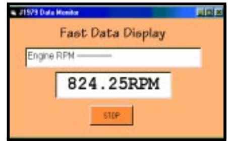
Photo 4 —The OBDScan Fast Data Display window is started by double clicking a data parameter. OBDScan software then samples the parameter as fast as it can (8 to 10 Hz), providing a real-time indication similar to a digital meter.
