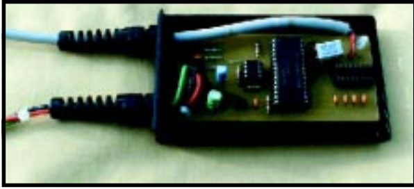
Photo 2 —Here's the completed and tested OBDScan Protocol Converter installed in a PAC-TEC case. The RS-232 cable is on top and the three-wire cable is the ISO-9141-2 interface.
