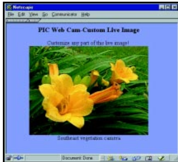
Photo 2—This is an example of the image presented by the PIC Web Cam's browser display. In this case, the image is automatically refreshed every 20 s, creating a live image.
