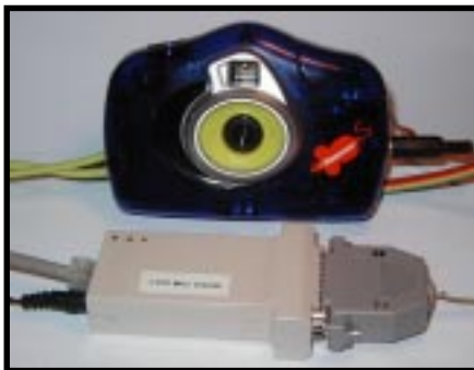
Photo 2 —The Nick Click camera is powered by the same 9-V supply as the PicoWeb. Plug this into your 10BaseT LAN and you can snap and display the photos with your favorite web browser.
