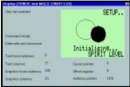
Photo 3—The LCD and display driver attributes allow the developer to easily see if the embedded program is functioning as expected.
