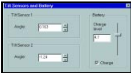
Photo 5 —Three separate threads, one for each sensor and one for the battery, service named pipes so that the A/D converter can retrieve suitably scaled values from this dialog box.
