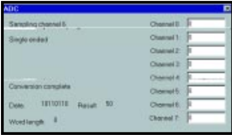
Photo 4 —The simulating A/D converter can fetch its inputs from the dialog box edit fields or from named pipes running anywhere else on the system.
