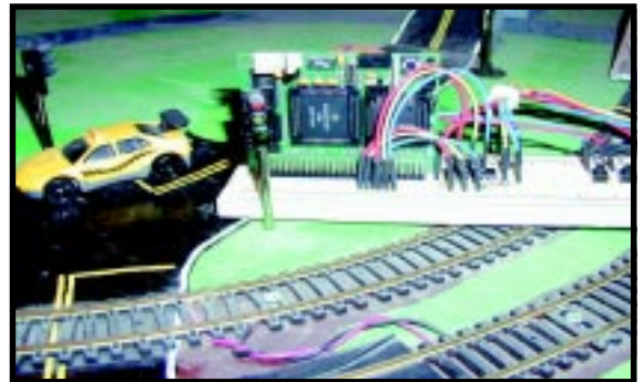
Photo 1 —A simulated traffic intersection is built with colored LEDs and is controlled by a Motorola MC68HC11.
