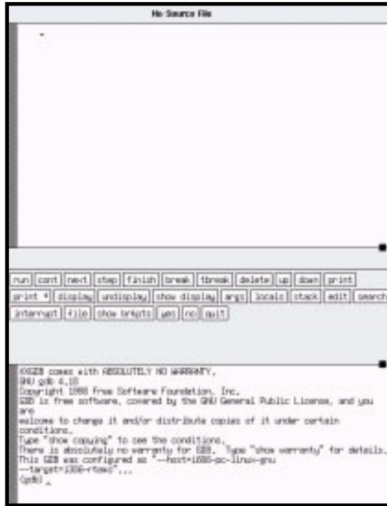
Photo 2 —Several GUIs exist for GDB to make it easier to use than the command line version. The sample that you see here is a simple X Window interface (xgdb).
