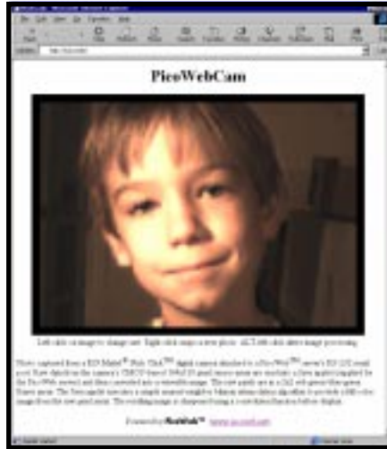
Photo 1 —The web page shows a photo that was captured by a Mattel Nick Click digital camera attached to a PicoWeb server's RS-232 serial port. Raw data from the CMOS-based 164 × 120 pixel sensor array are read into a Java applet (supplied by the PicoWeb server) and then converted into a viewable image. The raw pixels are in a 2 × 2 red-green-blue-green Bayer array. The Java applet uses nearest-neighbor bilinear interpolation to provide a full-color image from the raw pixel array. The resulting image is sharpened using a convolution function before display.
