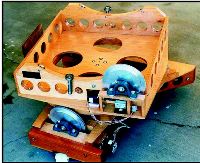
Photo 3—If one of the telescope mount's axes is pointed at the celestial pole, only that motor needs to turn at a constant rate.
