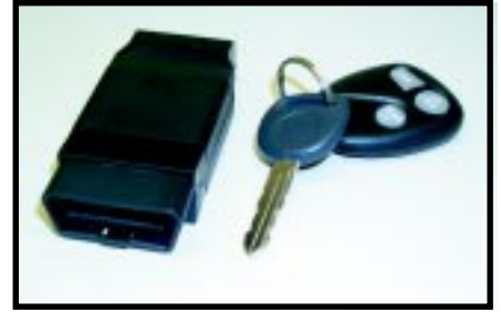
Photo 3—The Multiplex Engineering mux interface acts as a gateway between the vehicle network and anything with an RS-232 serial port.
