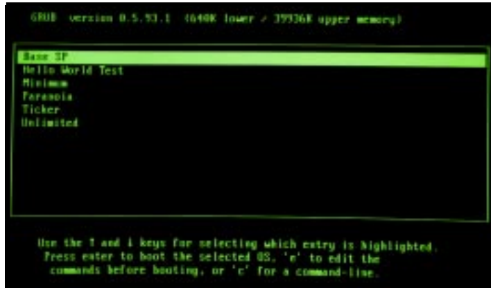
Photo 2—The boot menu displays a line for each application image. Highlight the one you want and hit enter. Grub can also be programmed to have a timeout value, after which it will boot a default.
