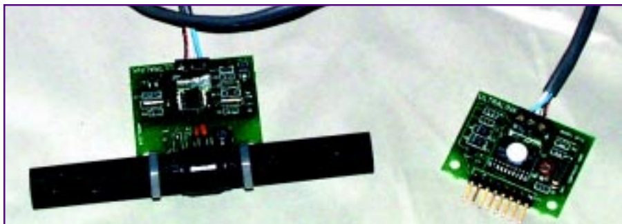
Photo 1 — The receiver unit contains all the analog circuitry to receive and demodulate the WWVB radio signal. The module also has a loopstick antenna.
