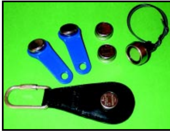
Photo 1 —Plastic key fobs as well as leather fobs and wallets will hold your iButtons. The probes are inexpensive and easy to connect. One wire is data and the other is ground. They can be mounted on any flat surface less than 10 mm thick.
