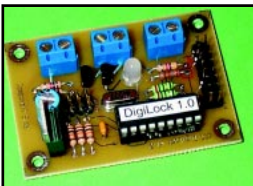
Photo 2 —The DigiLock board is small enough to mount almost anywhere. The iButton status bits are brought out via the 2 x 8 header. For security, locate the DigiLock where it cannot easily be tampered with. If it's outdoors, use a weatherproof box with a lock. If you have an alarm system, wire a tamper sensor inside the box to trip the alarm if anyone opens the box.
