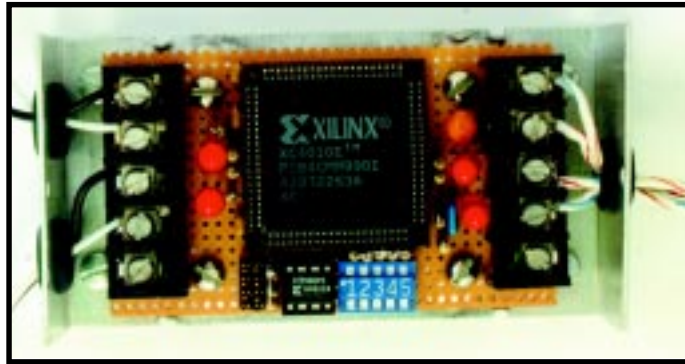
Photo 1 —An FPGA and serial PROM are the only active components in the completed design. The rest is DIP switches, status LEDs, decoupling caps, pullups, and connectors.
