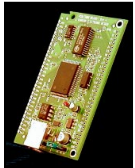
Photo 1 —The USBSIMM is a USB-enabled controller card that is placed in a 30-pin SIMM socket, or mounted vertically or horizontally on a board with 0.1" pin-center spacing.
