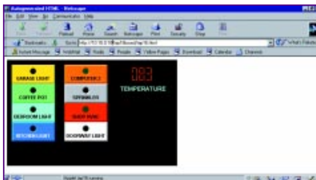
Photo 6—Okay, so it's 83° F outside. The little black hole in each of the switches is a status LED. The SHOP HVAC LED is green while all of the others are red.
