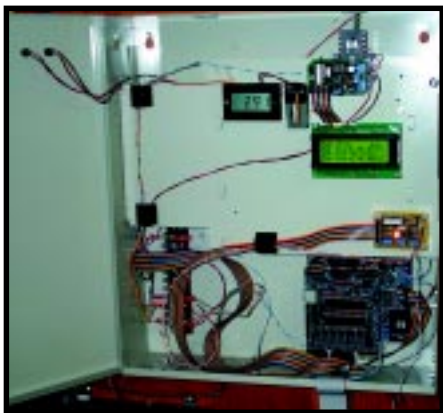
Photo 1 —Here's an LCD voltmeter monitoring the current draw of my remote nodes (and HCS-II boards on my test bench—thus the high reading). The boards in the cabinet are powered by a separate 5-V supply. The power resistor is on the lower left. A 3-W power resistor is more than adequate at 0.01 W.
