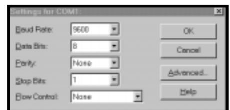
Photo 1—An example of a typical Windows dialog box used to configure serial port communications.
