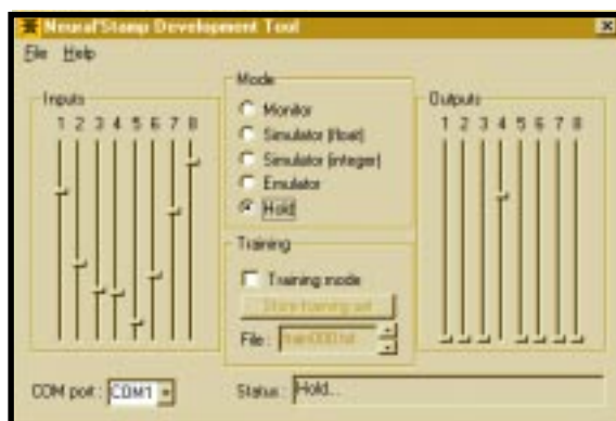
Photo 4—The neural network recognizes an input pattern close to the test case in C4 and indicates this with an active level on output 4.
