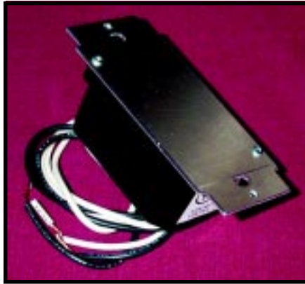
Photo 2—An X-10 signal bridge looks like a dimmer with no knob. You will need an extra deep, single-gang electrical box to install it in due to its size. Use 14/3 cable wired to a 15-A 220-V circuit breaker.
