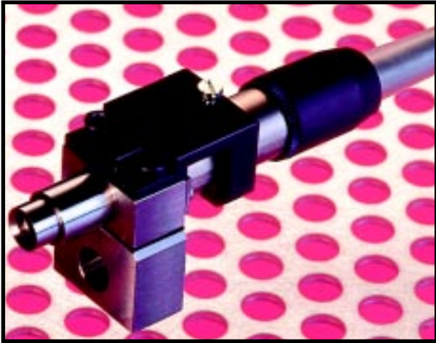
Photo 3—Laser position sensors have resolutions of 0.1 \mu\text{m} or better.
