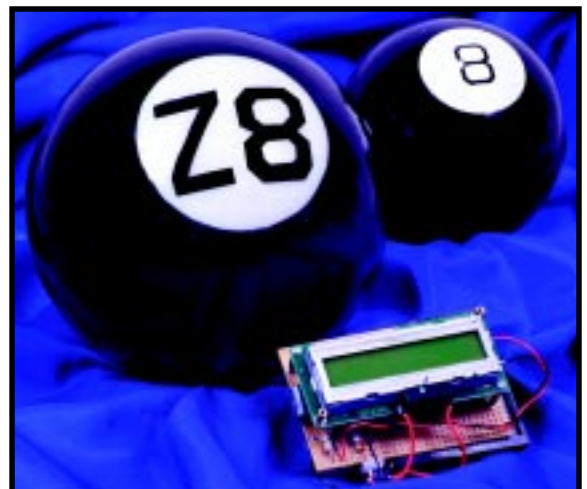
Photo 1 —I used a plastic ceiling globe for the Z8-ball. It's slightly larger than the original 8-ball. The circuitry is barely larger than the 1 \times LCD module.
