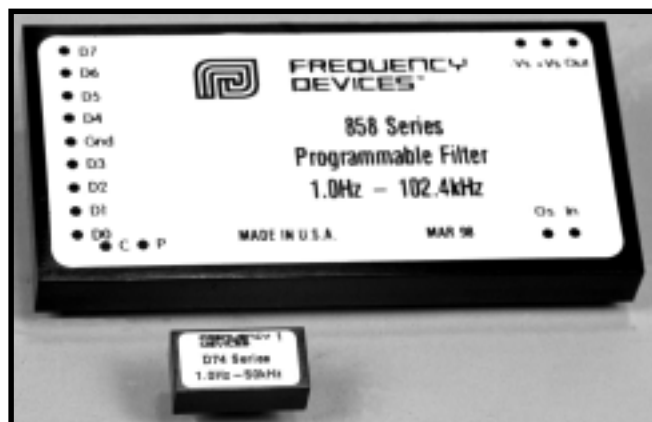
Photo 1 —These D74 and 858 series filter modules are manufactured by Frequency Devices.
