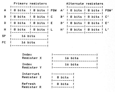
Figure 1.3. The Z-80 CPU registers.
