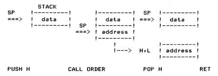
Figure 3.8. Improper mixing of data and the return address on the stack.
