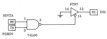
Figure 4.1. Circuit to convert an 8080 interrupt to an RST 5.
