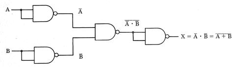
Figure 2.9. A NOR gate is obtained from four NAND gates.
