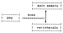
The CPU communicates with the user through such peripherals as the console, the printer, the disks, and so on. There are several electrical lines which are used to connect the CPU to the memory and to the peripherals. These lines are collectively known as the *buss*, or *bus*.
