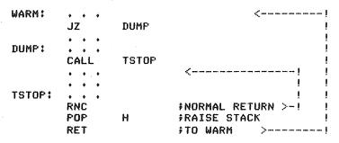
The stack pointer grows downward through memory during use. It is therefore common practice to place the stack as high as possible in available memory. But the system monitor may be located at the actual top of memory. In this case the stack can initially be placed lower in memory at the beginning of the monitor.
