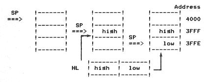
Figure 3.3. The HL register is pushed onto the stack.
