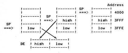
Figure 3.4. Two bytes are popped from the stack into DE.
