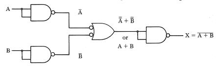
Figure 2.10. A NOR gate is produced from four NAND gates. The middle NAND gate is shown in its alternate representation.
