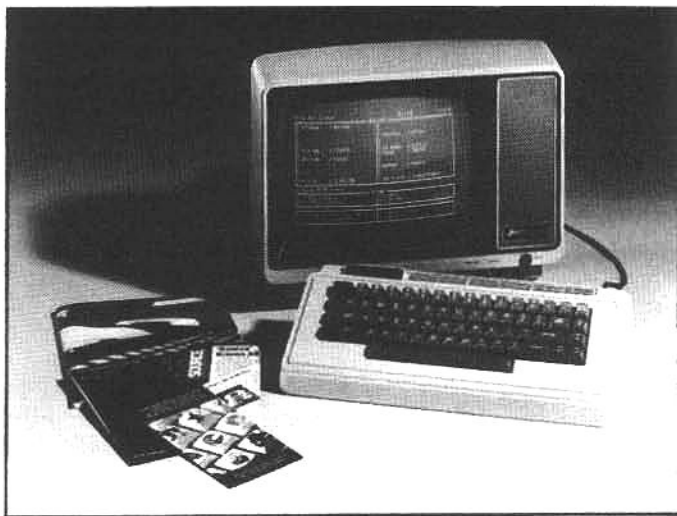
The Zenith ZT-1 is a sophisticated communications terminal with many features that make it ideal for remote "electronic mail" message transfer. Because of extensive built-in firmware, the ZT-1 can be "programmed" to perform automated tasks selected by the user from a menu display.
