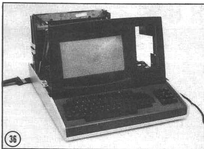
(36) The power is now applied to the computer, without the CPU board in place. This allows the user to verify power cable connections and to perform video board adjustments (to tune the CRT display). Note the screen display is too short and the background is not dark enough.
