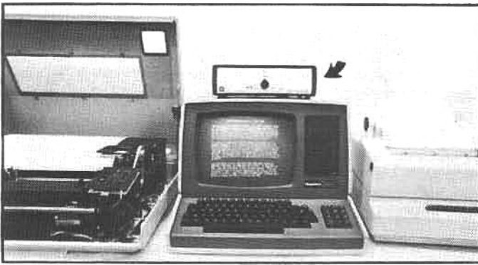
The Giltronix switch box (on top of the Z/H-89) can switch RS-232 serial data transmission between any of three devices. This system can send data to either the Z/H-25 on the left or the Siemens ink-jet printer on the right. The switch will operate with CP/M or HDOS.
