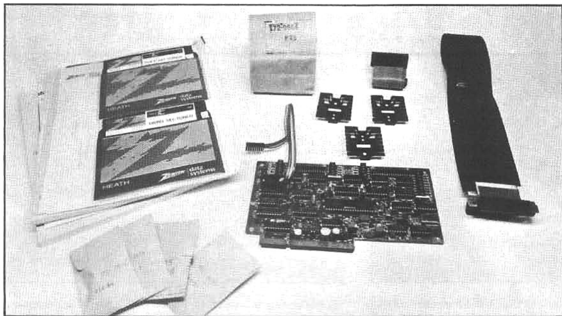
The Z/H-37 is a sophisticated upgrade that uses soft-sector storage structure to increase the amount of data that can be recorded on a 5.25-inch disk. If used with standard drives (replacing the hard-sector controller), the storage is almost doubled, and if used with Tandon double-sided drives, the storage space is expanded by a factor of six.
