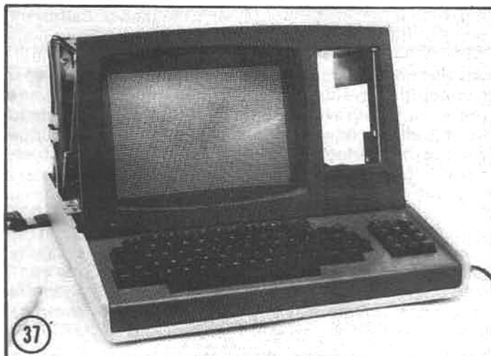
(37) After the adjustments on the video board have been completed properly the display fills the screen and the background (raster) is dark. So far...so good!
