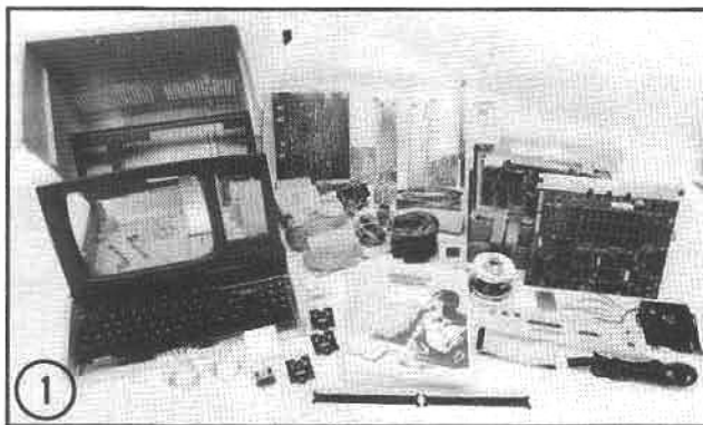
(1) The kit is complete with all of the parts required to build a functional H-89. Small parts—screws, nuts, resistors, etc.—are collected in brown paper bags to prevent loss. The bags are opened as needed, generally one for each subassembly.
