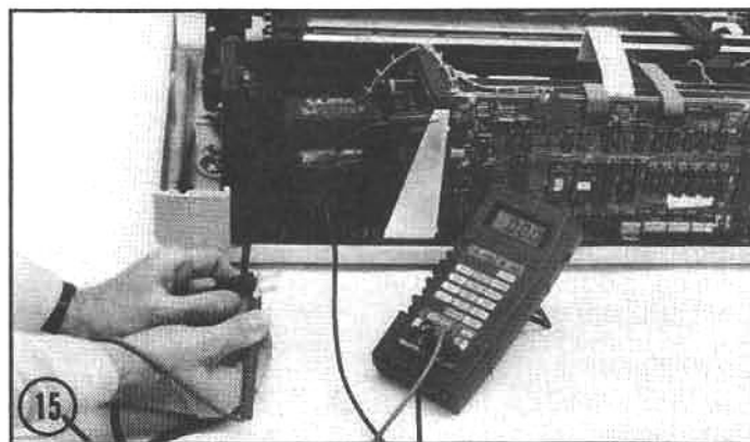
(15) When the power supply and cables are installed, the main circuit boards are slipped in place and the power supply lines are connected. At this point, a test (with an ohm meter) is performed to ensure proper wiring of the AC lines and circuit ground.
