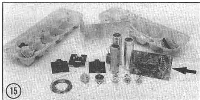
(15) The next project is the power supply. All of the components for this subassembly are located and organized (note that a plastic egg carton is being used to hold the small parts). The power supply is one of the three circuit boards (arrow) that must be assembled by the builder. It is a simple board to build.
