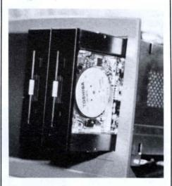
The solution to this problem is simple. File 1/16th of an inch off of the top and bottom of the lip around the floppy disk cutout on the H/Z-90. Mounting the drives in the H/Z-77 drive case is easily remedied without any case modifications by sliding the drives in from the rear.
