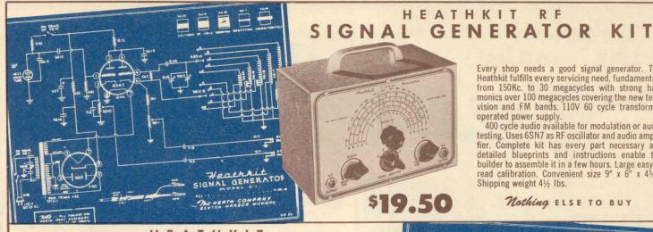
Every shop needs a good signal generator. The Heathkit fulfills every servicing need, fundamentals from 150Kc. to 30 megacycles with strong harmonics over 100 megacycles covering the new television and FM bands. 110V 60 cycle transformer
