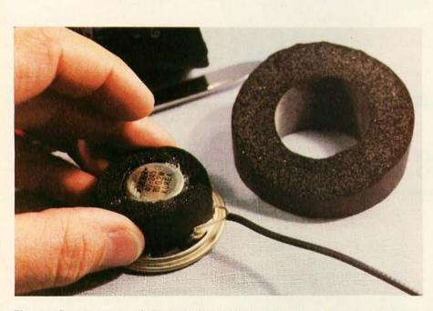
**Photo 3:** First of a series of photos (3 thru 9) showing how you can easily contruct an acoustic-coupler pickup. My design for the pickup uses such "exotic" materials as a hotwater pipe foam insulation, a pair of 2-inch, 8-ohm dynamic speakers, a foam-backed dinner placemat, rubber cement, and adhesive tape.
