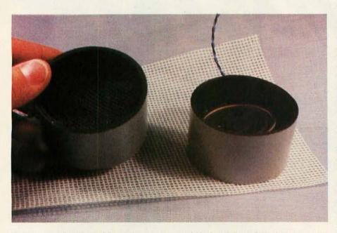
**Photo 8:** The final assembly can be spray-painted black as I have done, but this is not necessary. Caution: some paints act as solvents on foam and will produce a sticky mess. Test a small sample before spraying the whole unit, and don't spray the speaker cone.
