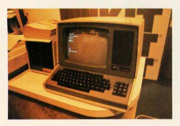
**Photo 1:** The Heath H-89, a Z80-based all-in-one personal computer with built-in 5-inch floppy-disk drive, WH-19 terminal, and 16 K bytes of programmable memory (expandable to 48 K bytes). The price for the assembled unit is \$2295.
