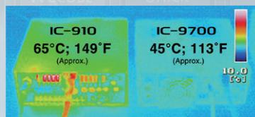
This is a comparison between two transceivers' rear chassis temperatures when continuously transmitting for 15 minutes. The IC-910\* rises to 65 °C while the IC-9700 rises only to 45 °C.
