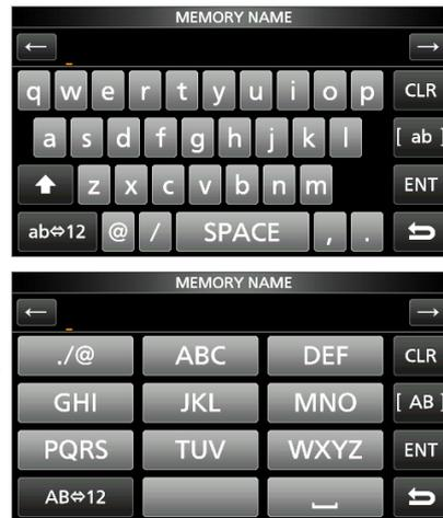
① You can select the full keyboard layout in “Screen Full Keyboard Layout” on the FUNCTION screen. (p.8-4)
