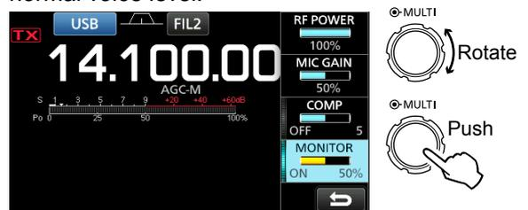
**NOTE:** When using the VOICE DELAY (p. 4-7), turn OFF the Monitor function. Otherwise the transmitted audio will echo.
