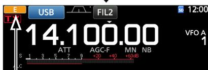
• The transceiver enters the Emergency mode (Tuner).
