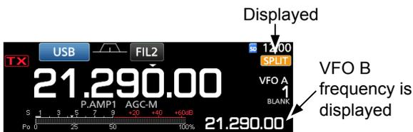
3. While holding down **[XFC]**, set the operating frequency offset between transmit and receive.
