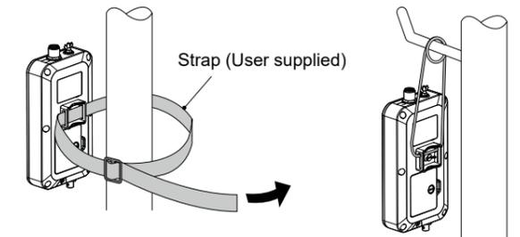
You can hang the antenna tuner, by threading a piece of cord through the bracket.
