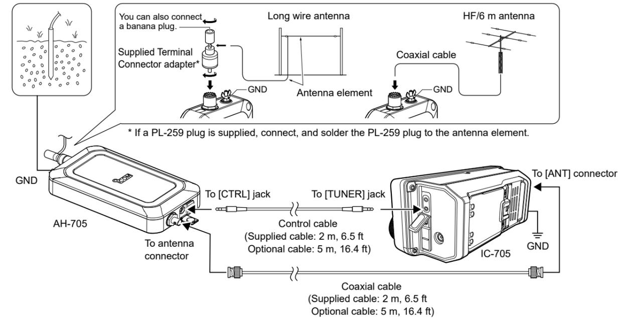
**NOTE:** The antenna tuner must have an adequate ground connection. Otherwise, the overall efficiency of the transceiver and antenna tuner installation will be reduced. Interference, RF feedback, and electrical shocks from other equipment could also occur.
