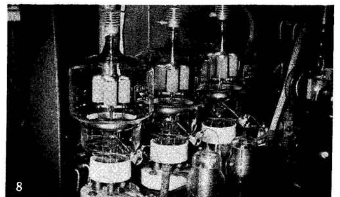
8 Eimac type 304TL tubes operating in a piece of flash brazing equipment. Two of these tubes are operated in class AB 1 in the audio driver stage of the 10-kw transmitter.
