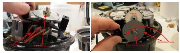
Step 8: Carefully slide the pot with Gears #1 and #2 (items #45 and #47) out from the Gear Box Plate, and pull the wires and the pot assembly out into the open.
