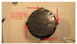
**Step 18:** Now keeping the Ring Housing raised up against the Upper Housing, squeeze the two together while flipping the rotor over onto it's top. Install the four 10mm bolts (item #4) through the Ring Housing into the threaded holes in the Upper Housing. Secure the bolts evenly and firmly into place, but do not over tighten!
