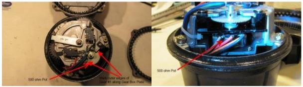
**Step 6:** Locate the 500 ohm position feedback potentiometer. It may be a good idea to mark the position of Gear #1 (item # 45) with a fine point marker to make it easier to see its position during reassembly. See the photo in this step, and in step 8.
