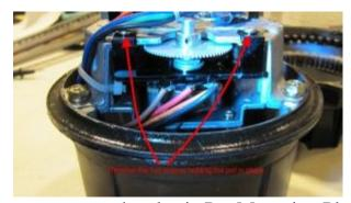
**Step 7:** Remove the two screws on the plastic Pot Mounting Plate (item #39) that hold the pot in place on the Upper Gear Box Plate Assy. (item #33).
