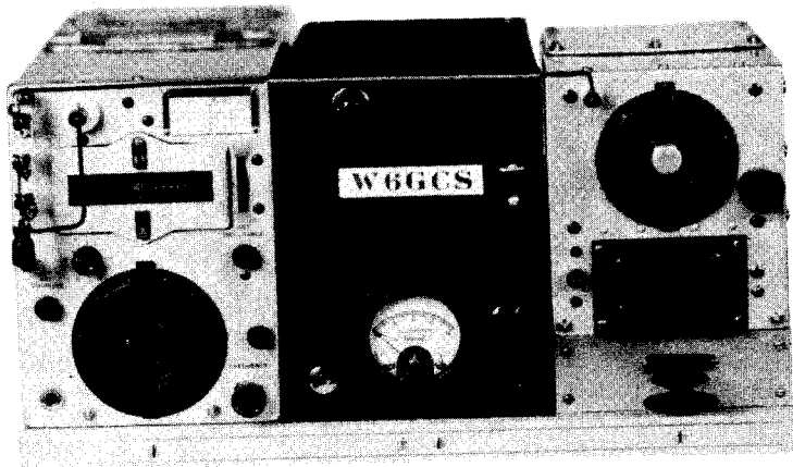
Fig. 1. The complete station. From left to right the units are: transmitter, a-c power supply, and receiver. The hand key is mounted underneath the receiver.
