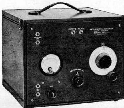
A piezo-electric oscillator, a device which maintains constancy of frequency
