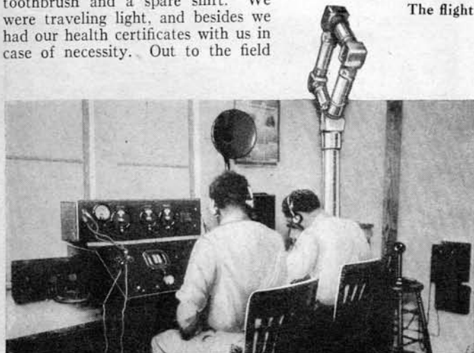
Pan-American radio headquarters WKDL at Miami, Florida. The loop is used for bearings on the six hundred meter to eight hundred meter band
