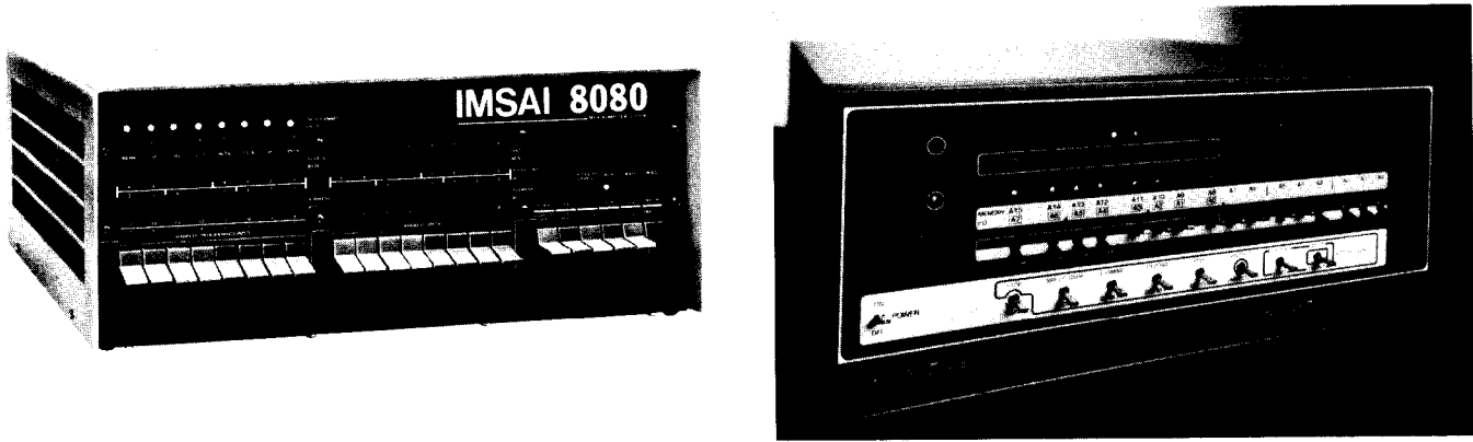
Fig. 1.9 The heart of any computer system, the computer itself, typically comes in a large case with many front panel switches and indicators. The Imsai 8080 (left) and the Pertec Altair 8800b (right) were two of the first personal computer systems. (Courtesy Pertec and Imsai)
