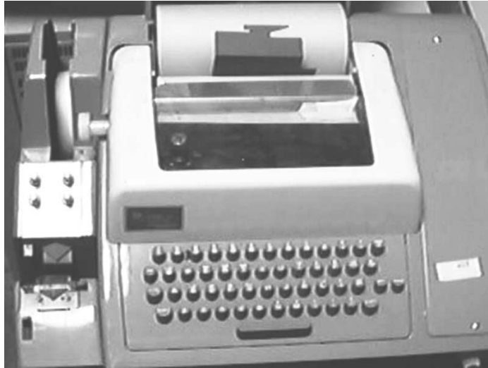
Figure 17-1. A teletype incorporated a keyboard and a printer into a single terminal
