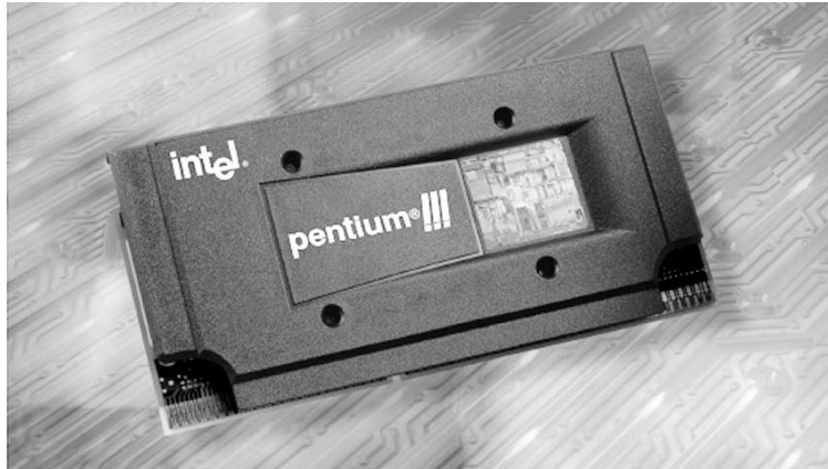
Figure 3-20. The Pentium III processor in the Slot 1 SECC2 package. Photo courtesy of Intel Corporation
