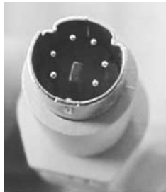
Figure 18-17. A 6-pin mini-DIN (PS/2) connector is standard on most PC keyboards
