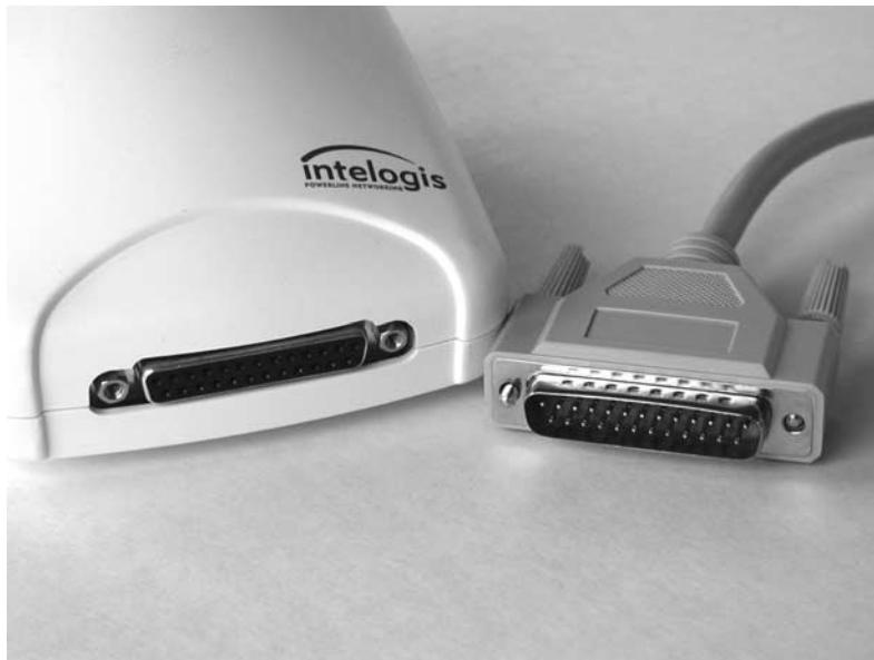
Figure 19-7. A networking device with a parallel port and a cable with a DB-25 male connector
