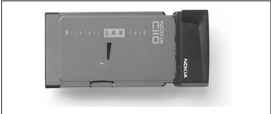
Figure 20-14. An 802.11 (WLAN) PCMCIA Type II network adapter card. Photo courtesy of Nokia
