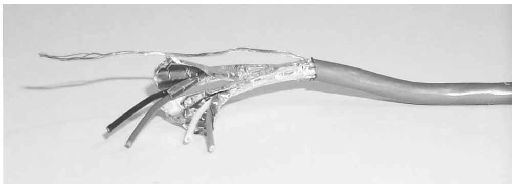
Figure 20-6. The foil wrapper of shielded twisted pair (STP) cable
