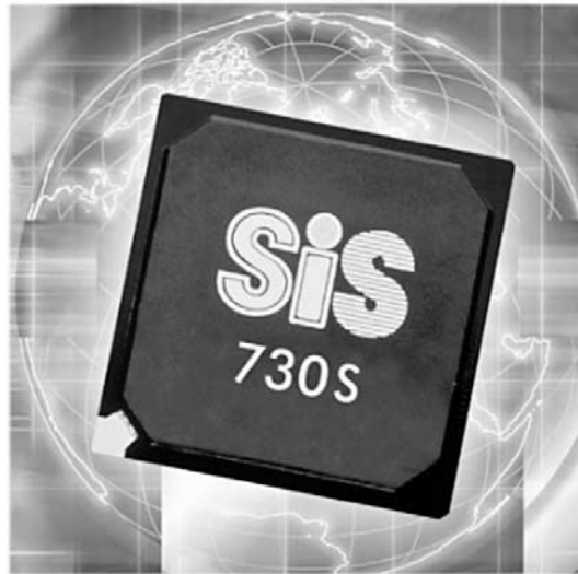
Figure 5-9. The SiS 730S single-chip chipset. Photo courtesy of Silicon Integrated Systems Corporation
