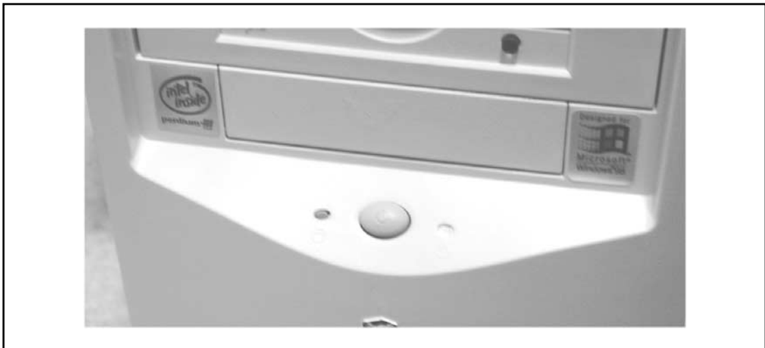
Figure 15-7. The power and reset switches on a PC front panel
