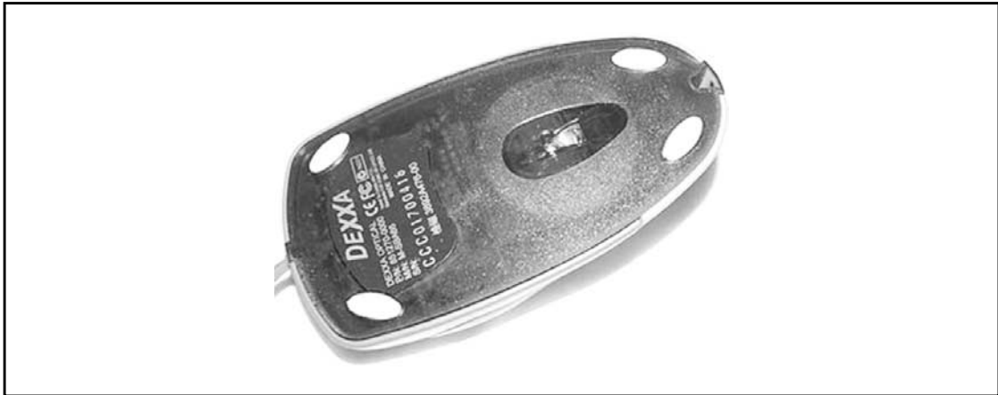
Figure 18-24. The business side of an optical mouse. Photo courtesy of Logitech, Inc.
