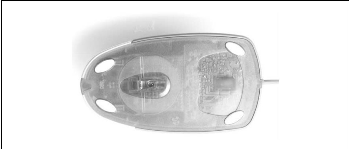
Figure 22-4. An optical mouse, which does not have a ball or moving rollers and sensors, eliminates most of the cleaning required for a ball mouse
