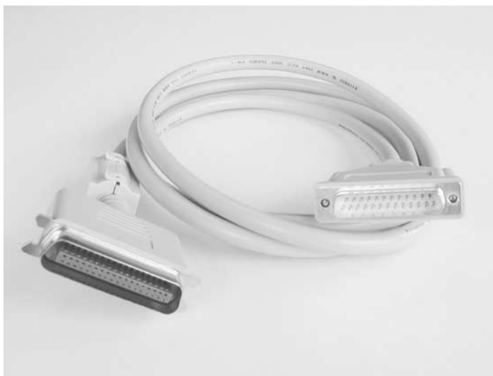
Figure 17-2. A printer cable with a 36-pin Centronics head on one end and a DB-25 connector on the other
