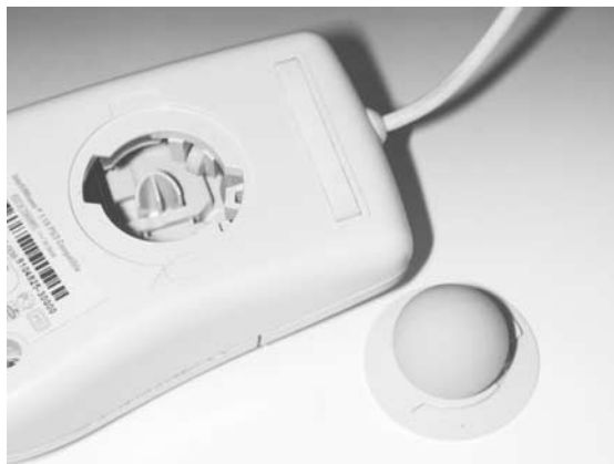
Figure 22-6. The mouse ball chamber must be inspected for lint, dirt, and other debris
