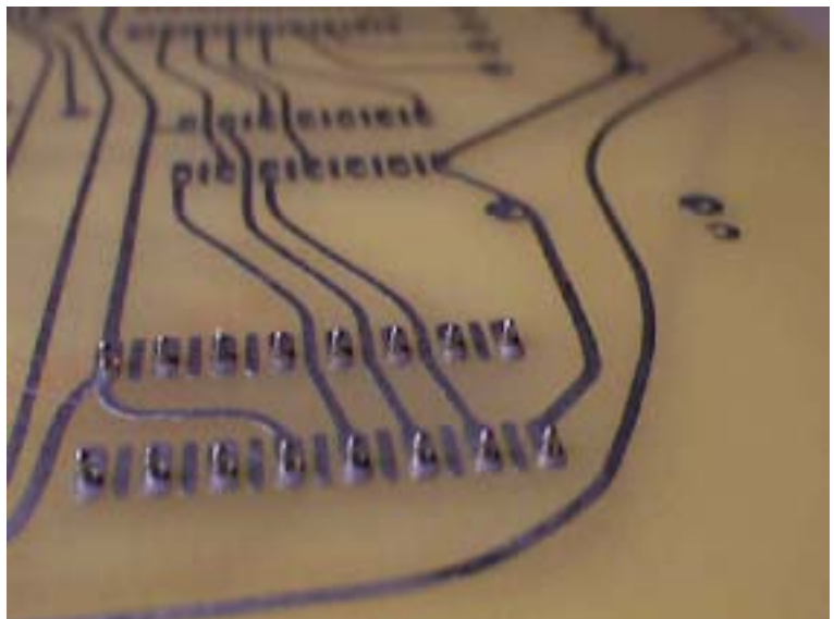
Figure 9 Bottom View of Properly Installed Socket
