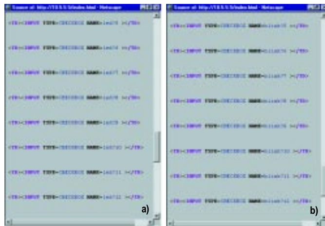
Photo 4a—None of the checkboxes are CHECKED here and thus none of the LEDs are On. The CHECKED attribute is returned with the served page to put a check in the browser boxes. b—Basically, this is the same logic and HTML that applies in (a). The names have been changed to protect the innocent.
