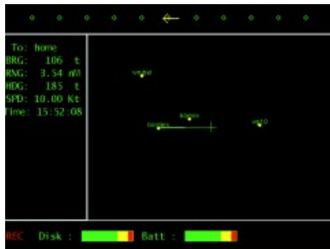
Photo 3—To the left in this GUI is pertinent navigation information (e.g., heading, speed and bearing, distance to the next waypoint). At the top is the course deviation indicator. The needle indicates the direction to turn, and the horizontal mark is the cross-track error. Keep the needle straight and in the middle, and you'll fly right over the destination waypoint.
