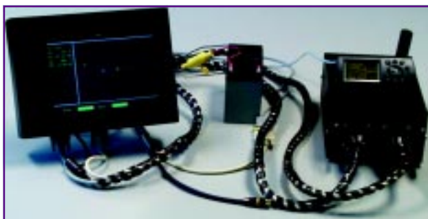
Photo 2—Here you see the computer box, the battery, display, and external GPS receiver. The computer is a ruggedized EBX module with a PC/104 stack. The display is a daylight-readable 8.4" LCD flat-panel with touch-sensitive screen.
