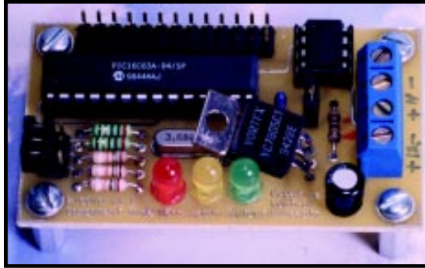
Photo 1 —The simple PIC-DIO hardware allows for quite a small circuit board. Imagine if you used surface-mount devices!
