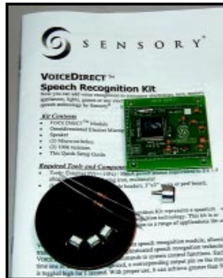
Photo 2 —The kit includes the module, resistors, three push-button switches, microphone, speaker, and manual—all the external components you need to implement stand-alone recognition.
