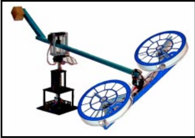
Figure 1 —The helicopter model consists of two motors driving two propellers mounted on a frame that can freely pitch. The frame is mounted on a long arm with a counterbalance. The entire arm can pivot and elevate, resulting in three degrees of freedom of movement.
