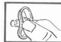
2. AFTER DISCHARGING THE VOLTAGE, DISCONNECT THE ANODE LEAD FROM THE CRT.
