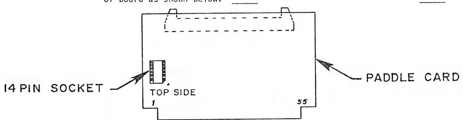
The assembly of the paddle card is now complete with the exception of the IC. At this time there should be NO IC plugged into the socket. Visually inspect your board for missed or cold solder joints. After the inspection, with everything checking out, install the I.C..
