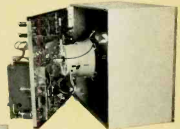
Vertical Swing-Out Chassis! Makes chassis more accessible for servicing and installation.
