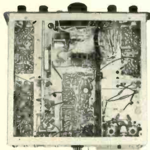
Sectionalized layout on circuit boards simplifies construction—makes components accessible and easy to locate.
