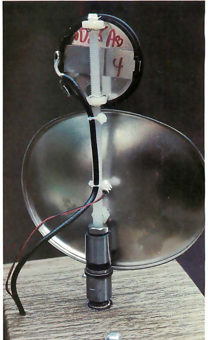
Photo 8: Close-up of the back side of the reflector and transducer of the scanner, showing the mounting apparatus.
