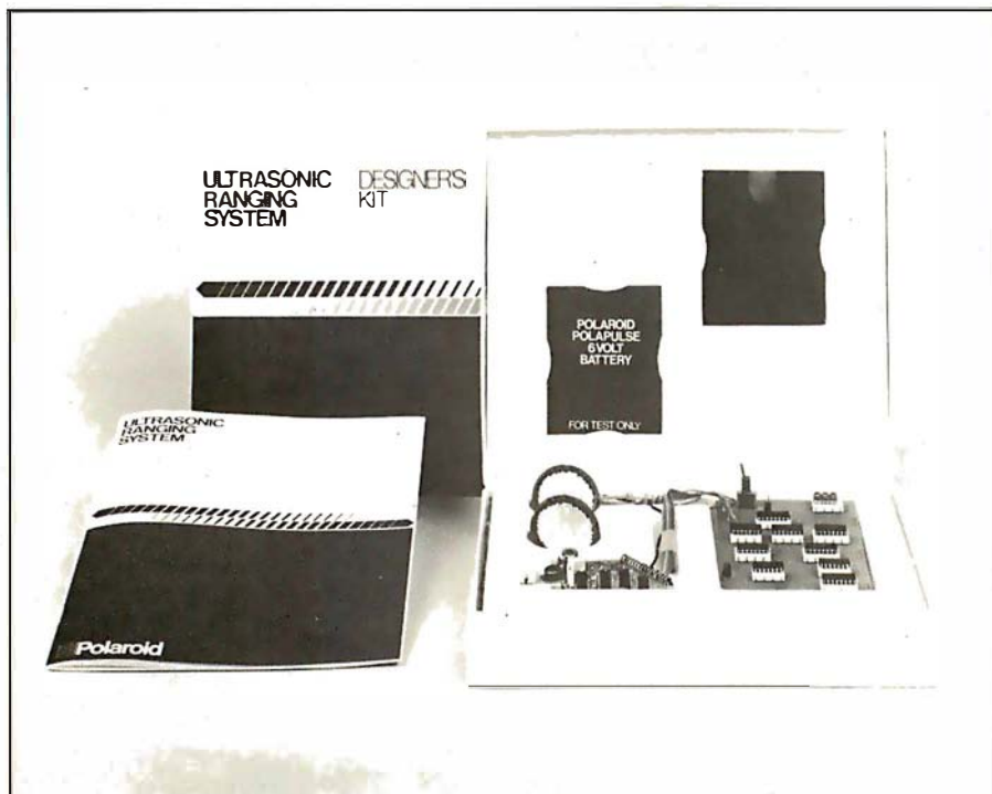
Photo 2: Polaroid Ultrasonic Ranging System Designer's Kit, which includes ultrasonic sonar transducers, electronic circuitry, and a detailed specifications booklet.
