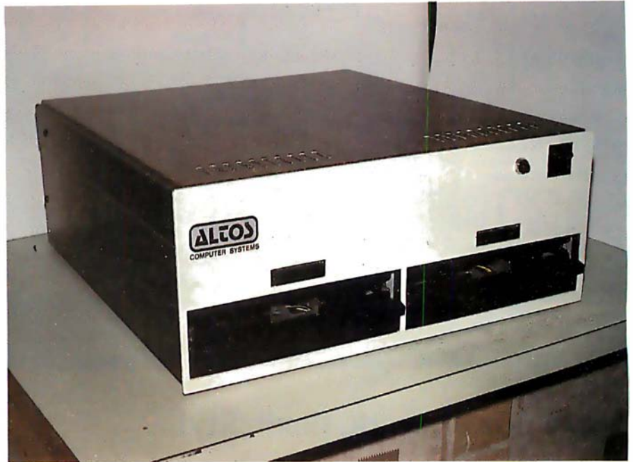
Photo 1: Front view of the Altos ACS 8000-2 computer, which has 64 K bytes of memory and two dual-density, single-sided disk drives.
