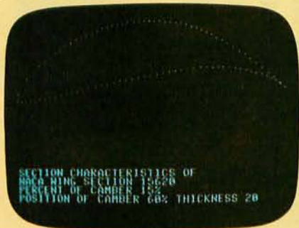
Apple's existing software library includes a program that plots the shape of an airfoil, given its parameters.
