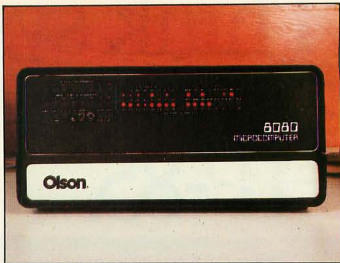
Photo 3: Assembled front panel for the 8088-based computer. Two toggle switches and a push-button switch have been added to the LED assemblies shown in photo 2.
