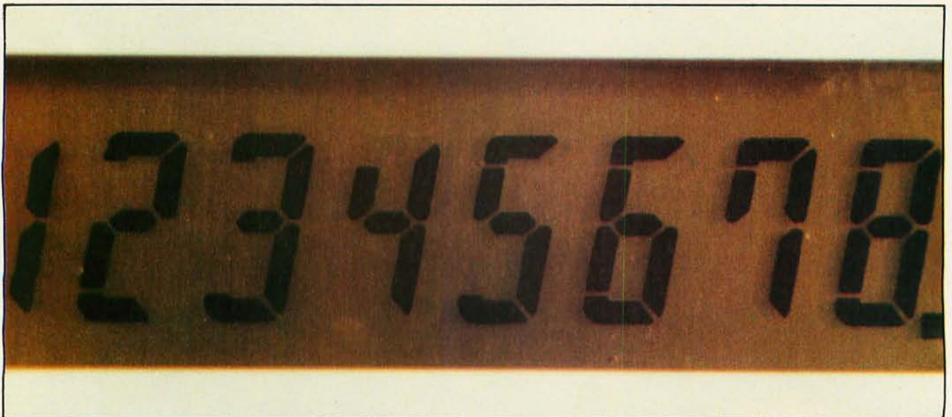
Photo 8: Typical eight-digit, seven-segment LCD calculator display.
