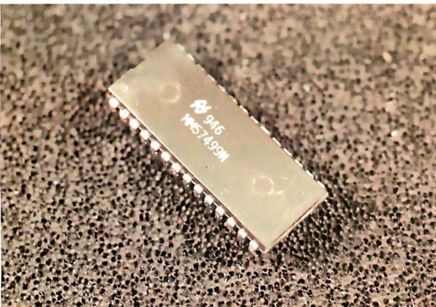
Photo 4: This twenty-eight-pin integrated circuit keeps things simple by performing the keyboard encoding and transmitting resulting data serially. It also takes care of display functions, with the addition, in figure 2a, of a single shift register.
