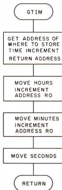
Figure 4: Flowchart of routine that reads the clock.
