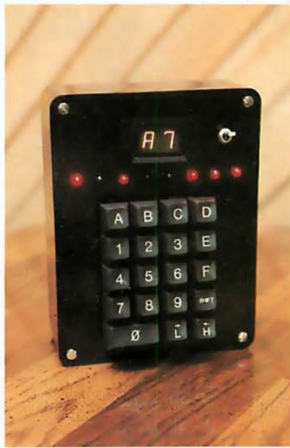
Photo 2: The remote data-entry terminal. Using a new serial keyboard-interface integrated circuit, construction is simple and inexpensive.
