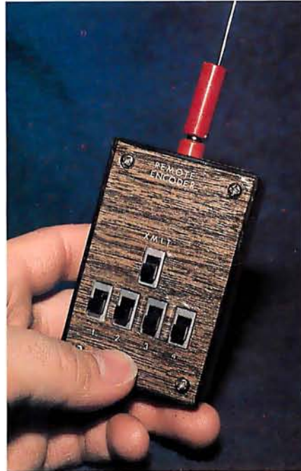
Photo 1: The handheld biphase FSK remote-control transmitter, which uses the circuit shown in figure 3. The transmit (XMIT) switch is a momentary power switch; the other four switches are used to set a 4-bit control-channel code.
