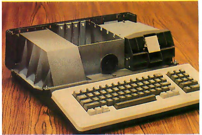
Photo 3: The Apple III with its plastic case removed to reveal the shielded aluminum chassis, designed for heat dissipation and RFI (radio-frequency interference) containment.
