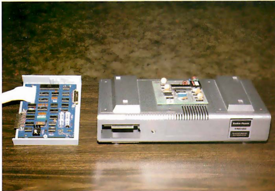
Photo 2: Here are two ways of adding RS-232 communication capability to the Radio Shack TRS-80. The COMM-80 unit is shown on the left; the combination of the Radio Shack expansion interface and serial-interface board is shown on the right.
