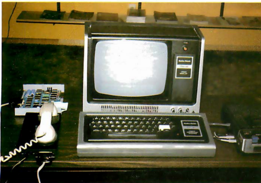
Photo 3: A TRS-80 equipped with Level II BASIC, the COMM-80 interface, and a Novation CAT modem can be used as a remote terminal for a time-sharing service such as the Source.
