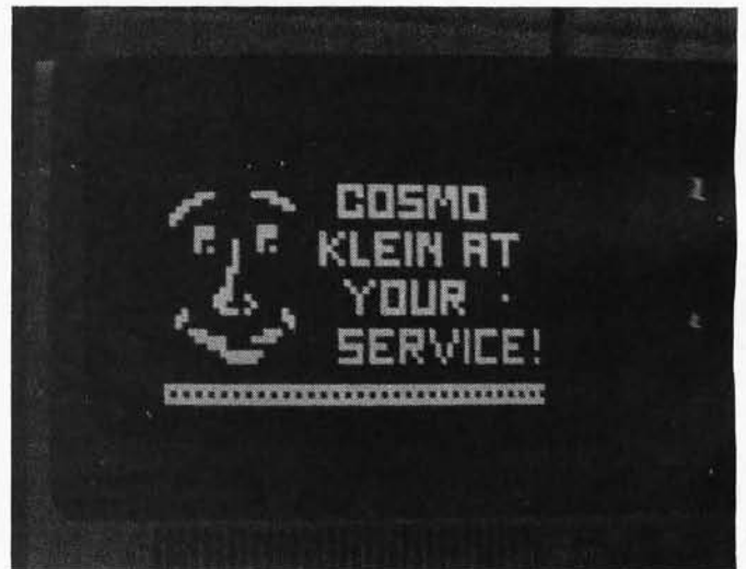
Photo 4: Display produced using the Video Doodler. The isolated dot at the center right is the winking cursor.
