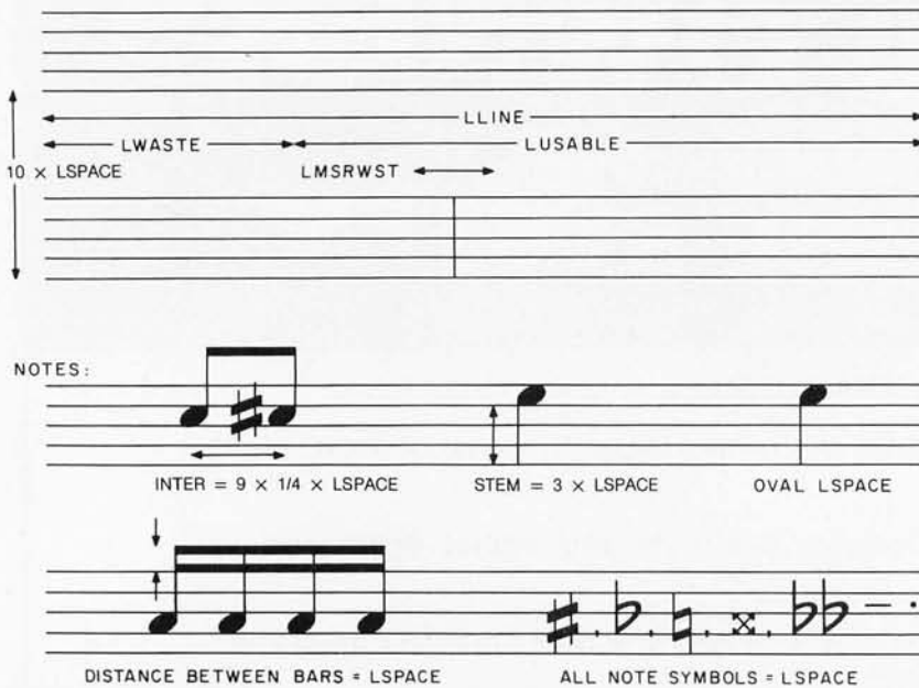
Figure 5: Dimensions of the musical staff, notes, and symbols. All dimensions are given in terms of LSPACE, the distance between the lines of the staff.
