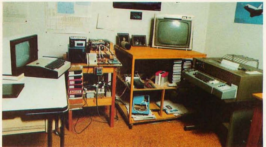
Photo 1: The author's personal computer system. It contains the following commercially built equipment: a MOS Technology KIM-1 microcomputer, three 8 K-byte Digital Group static memory boards, a Percom LFD-400 floppy-disk controller and two Shugart 5-inch floppy-disk drives, a Southwest Technical Products Corporation GT-6144 graphics board, an ACT-IA terminal with Leedex monitor, an Olivetti TE-300 hard-copy terminal, and several Lambda power supplies. Homebrew equipment in the system includes a programmer for erasable programmable read-only memories (EPROMs), a programmable integrated-circuit tester, a calculator interface, the motherboard, and the input/output (I/O) interface board.
