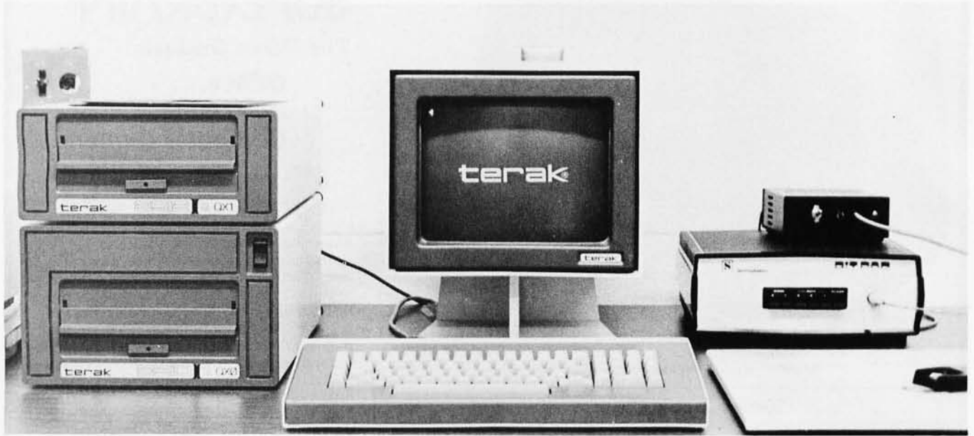
Photo 1: The Terak microcomputer with dual floppy-disk drive, video display, and keyboard. The Summagraphics Bit Pad consists of the digitizing tablet and the microcomputer control unit.
