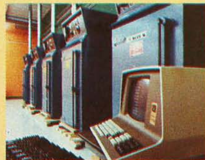
For high reliability all Cromemco memory cards are burned in at the factory in these temperature-controlled ovens.
