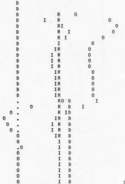
Figure 13: A look at different reference signal effects. As explained in the text, the disturbance signal has made the perceptual signal match the reference signal.
