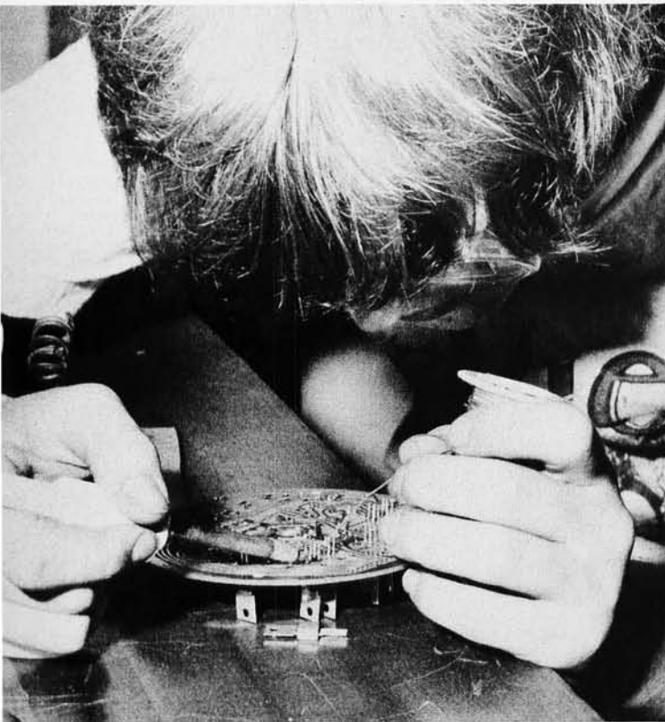
Photo 4: Soldering the installed components.
