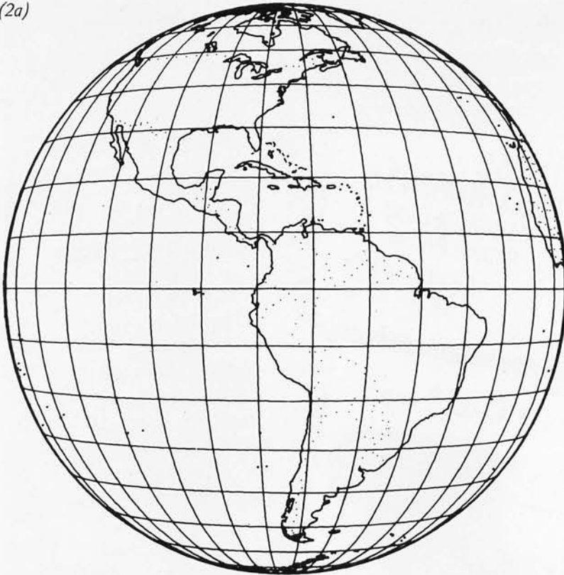
VIEWED FROM 35862 KM OVER 0:00N 75:00W. FACING 0 DEG AZIMUTH PERSPECTIVE PROJECTION PREPARED BY WILLIAM D. JOHNSTON
