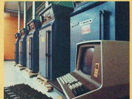
For high reliability all Cromemco memory cards are burned in at the factory in these temperature-controlled ovens.
