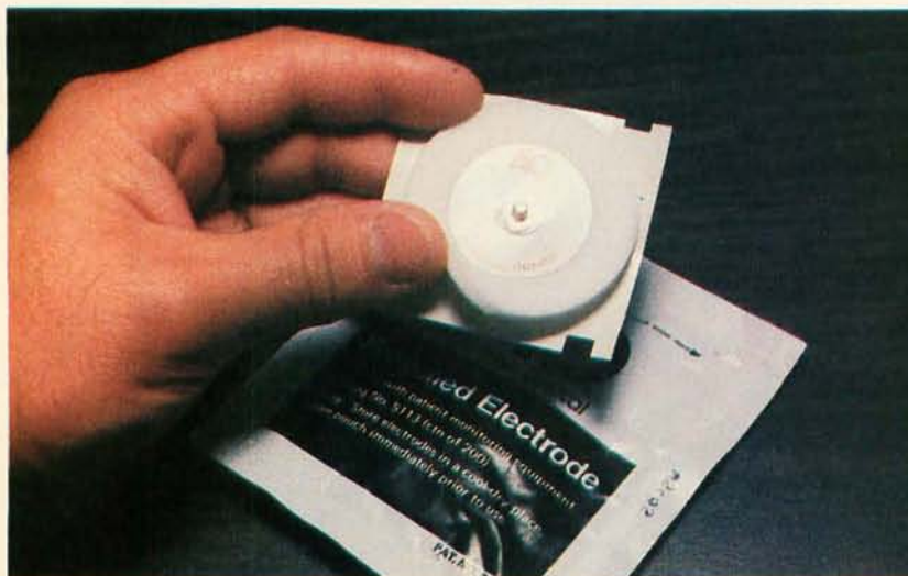
Photo 4: Pregel American Optical electrodes of the type used in this article. They are available from medical supply outlets.
