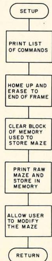
Figure 2: Flowchart expansion of setup block from figure 1.
