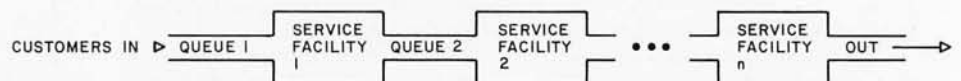
Figure 4: Single queue multifacility system, in which the customer waits in a queue to use a facility, then waits in another queue for the second facility, and so on until all service facilities have been used.
