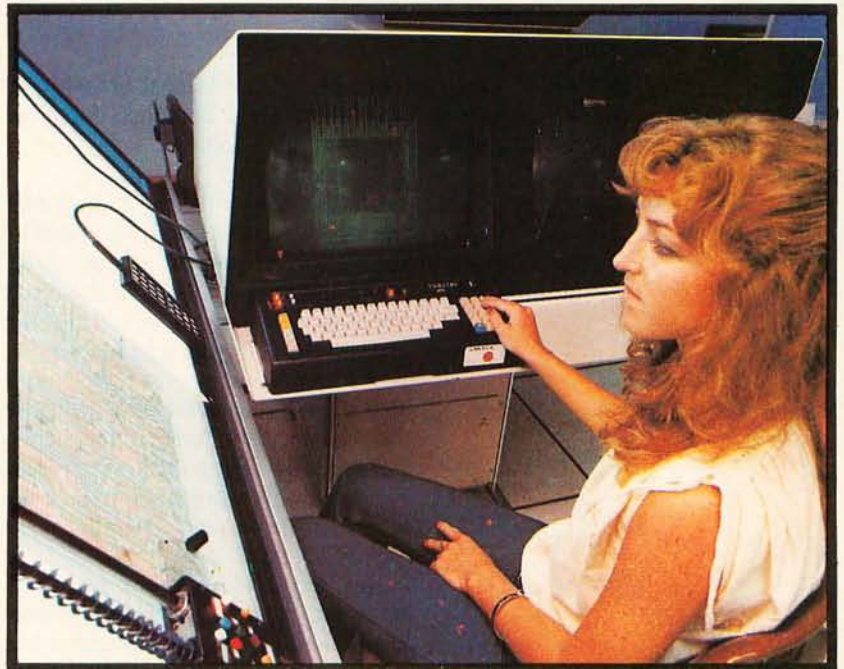
Photo 4: Digitizing. Computer aided design (CAD) technician Lisa Fink enters a cell layout into the data base. The cursor on the light table is used to transfer precision measurements to the computers. An already digitized cell is shown on the video display.
