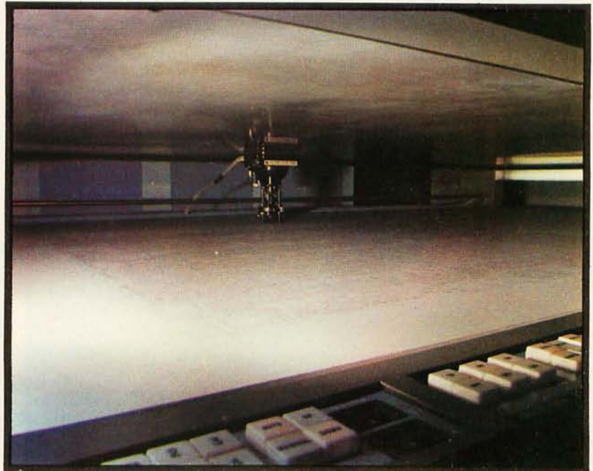
Photo 3: Plotting the circuit layout. Huge precision plotters display the computer data base which will become the chip. The layout plot is then checked by circuit engineers both for proper interconnection and exact transistor sizing. Any problems thus uncovered will be repaired by editing the data base.
