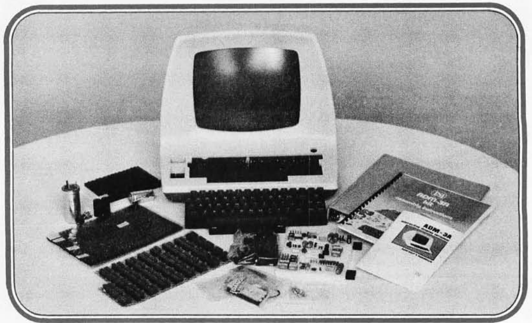
Photo 1: Lear Siegler ADM-3A "dumb" terminal kit. When the kit is unpacked, the various parts are grouped in convenient sections.
