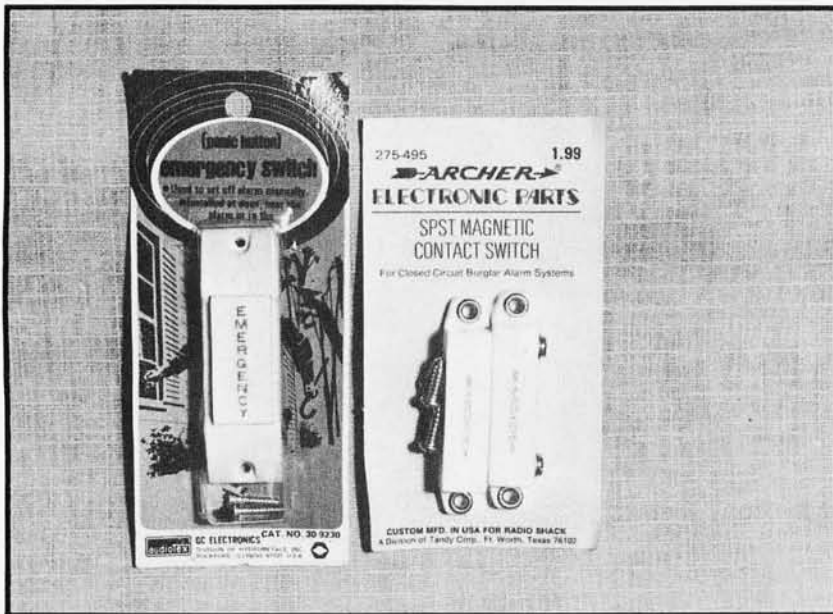
Photo 4: Typical commercially available sensors. Shown are a panic button (left) and magnetic door switch, available from GC Electronics, Rockford IL, and Radio Shack, respectively.
