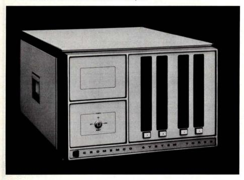
Cromemco's System Three is ideal for a wide range of professional work in almost any field. It consists of a 4 MHz Z-80 based microcomputer, 32 K bytes of programmable memory (two 16 K byte cards) expandable to 512 K bytes,
