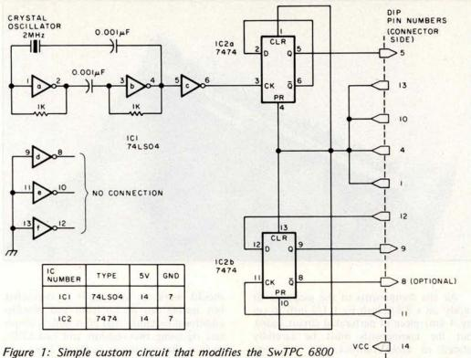
Figure 1: Simple custom circuit that modifies the SwTPC 6800 computer so the user can change the processor clock speed by plugging in different crystal oscillators. The entire circuit can be mounted on a small perforated circuit board (see photos 1 and 2) which plugs directly into the SwTPC 6800 board in place of the existing 7474 data rate generator timebase divider.
