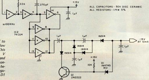
Figure 2: A CMOS DC to DC converter used for low current applications. This circuit produces -15 V from a +15 V source and provides a relatively constant output voltage because of the shunt regulator formed by diodes D1 and Q1.
