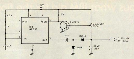
Figure 3: A variable output DC to DC converter capable of producing 0 to -10 V.
