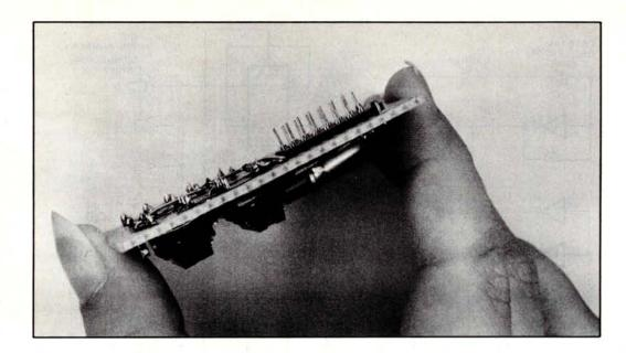
Photo 2: Side view of the clock modifier circuit, showing the pins of the dual in line connector (DIP) plug, enabling the experimenter to plug the entire board into the SWTPC board in place of the existing 7474 flip flop, which serves as the data rate generator timebase divider.
