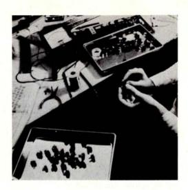
Photo 4: After soldering the switches to the keyboard printed circuit board, each switch must be individually tagged with a preprinted self-sticking key identification. The key identification fits into a recessed flat area on the upper side of the keytop.
