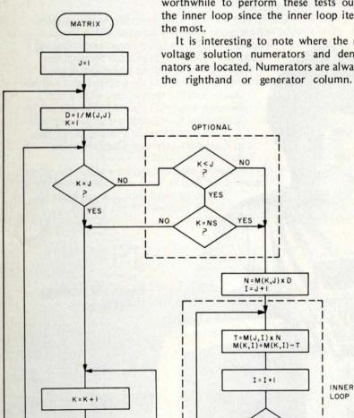
nominators are always in the main diagonal from upper left to lower right. Row position is equal to node of solution. Highest node numerators and denominators are always found; back solution is required only for nodes less than the highest node. The back solution algorithm is called the Gaussian elimination or Gauss-Jordan method of solution.
