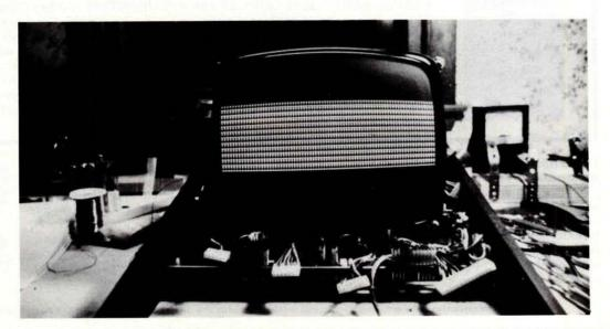
Photo 2: Several steps later in the manual, the deflection yoke has been carefully twisted around the neck of the cathode ray tube to produce horizontal rows of null ("?") characters.
