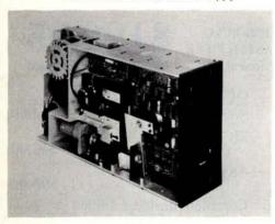
This 4 headed flexible disk drive stores up to 3.2 M bytes of data in the space required by a standard size floppy drive. The new PerSci Model 299 diskette drive interfaces to microcomputers using the 8080, 6800, or Z-80 processors, as well as minicomputers.
