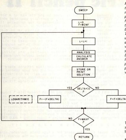
Figure 7: The SWEEP routine, used to perform a number of analyses on a particular circuit over a frequency range. Two types of sweeps are possible: linear and logarithmic. The variable DELTA is used as an increment and also as an indicator of which type of sweep analysis is to be performed. If DELTA is negative, a logarithmic analysis will be performed; if DELTA is positive, a linear analysis will occur.
