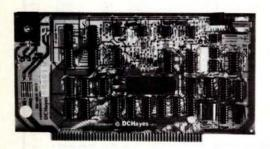
This 80-103A Data Communications Adapter has been developed to function as a S-100 bus compatible serial interface
