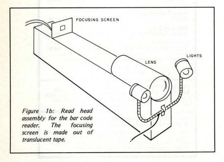
to a base. This allows us to move the read head up and down while keeping it level.
