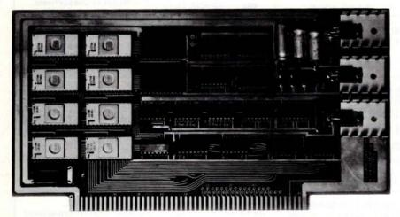
This programmable read only memory (PROM) board for the S-100 bus can be used with eight 2708 type E read only memories with provisions for using
