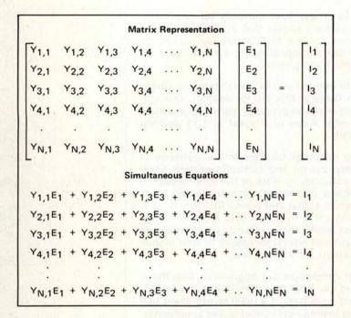
Figure 2: Matrix and simultaneous representations of any circuit. In the figure, and also in the text, the following conventions hold:
