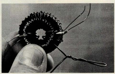
Photo 5: The completed transformer. The ends of all enameled wires should be cleaned of insulation before soldering.
