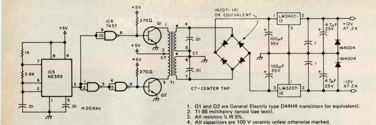
Figure 5a: 5 W DC to DC converter pictured in photo 1, which produces 0.2 A at +12 and -12 V from a 5 V source. See figure 5b for details of winding a toroidal transformer for this circuit.
