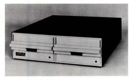
The Southwest Technical Products Corp DMAF1 is a dual drive, single density, double sided 8 inch floppy disk system. The hardware consists of a SS-50 bus (SwTPC 6800) compatible direct memory access controller capable of handling up to four drives, two CalComp 143 M double density rated disk drives, 5 3/4 by 17 1/8 by 20 1/2 inch (14.5 by 43.5 by 52 cm) aluminum chassis, regulated power supply, drive motor control board, cooling fan, diskette and interfacing cables.
