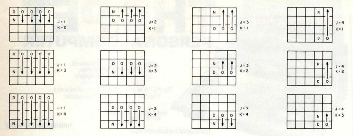
Figure 5: Sequential solution for all nodes of a 4 node circuit. This solution is the type that would take place if the optional section of figure 4 were deleted.
