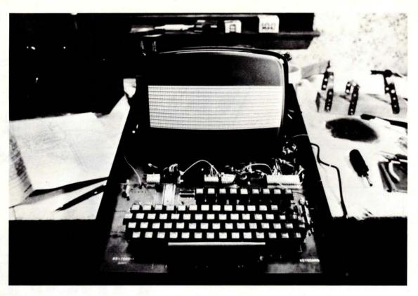
Photo 6: After installation of the keyboard, another live test of the display is performed, this time using the keyboard to vary the content of the display.
