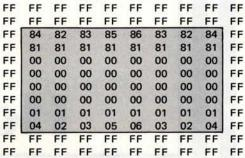
Figure 3: Representation of the pieces on their home squares. Pieces are identified by means of unique byte values.
