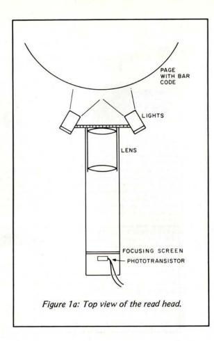
The phototransistor was mounted peeking through some translucent tape which served as a focusing screen. The entire assembly was covered on the top and sides with a cardboard hood to exclude ambient light. The block of wood on which the read head was assembled was attached to two strips of wood, which were in turn attached
