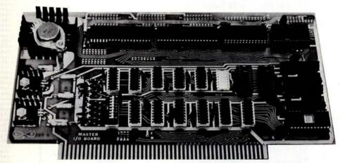
The Master IO contains enough read only memory and IO to allow a 2 board S-100 system and can be used to emulate the Intel SBC IO functions. This board can replace a real time clock, a fre-
