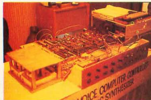
Photo 7: Homebrew 3 voice computer controlled music synthesizer built by John Pratt and Don Shertz of Monterey CA.
