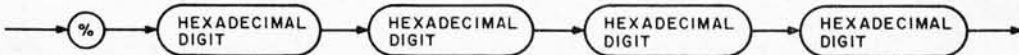
Figure 3, continued: Elementary constructs for Pascal subset. Hexinteger is usually not defined in Pascal but is used here so that actual memory locations can be easily manipulated.
